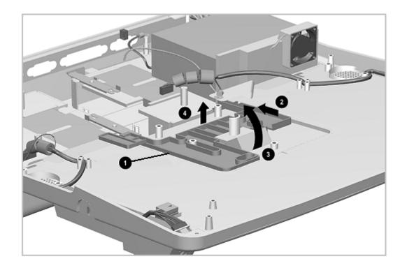
Figure 7-37. Removing the Puller Plate Assembly
